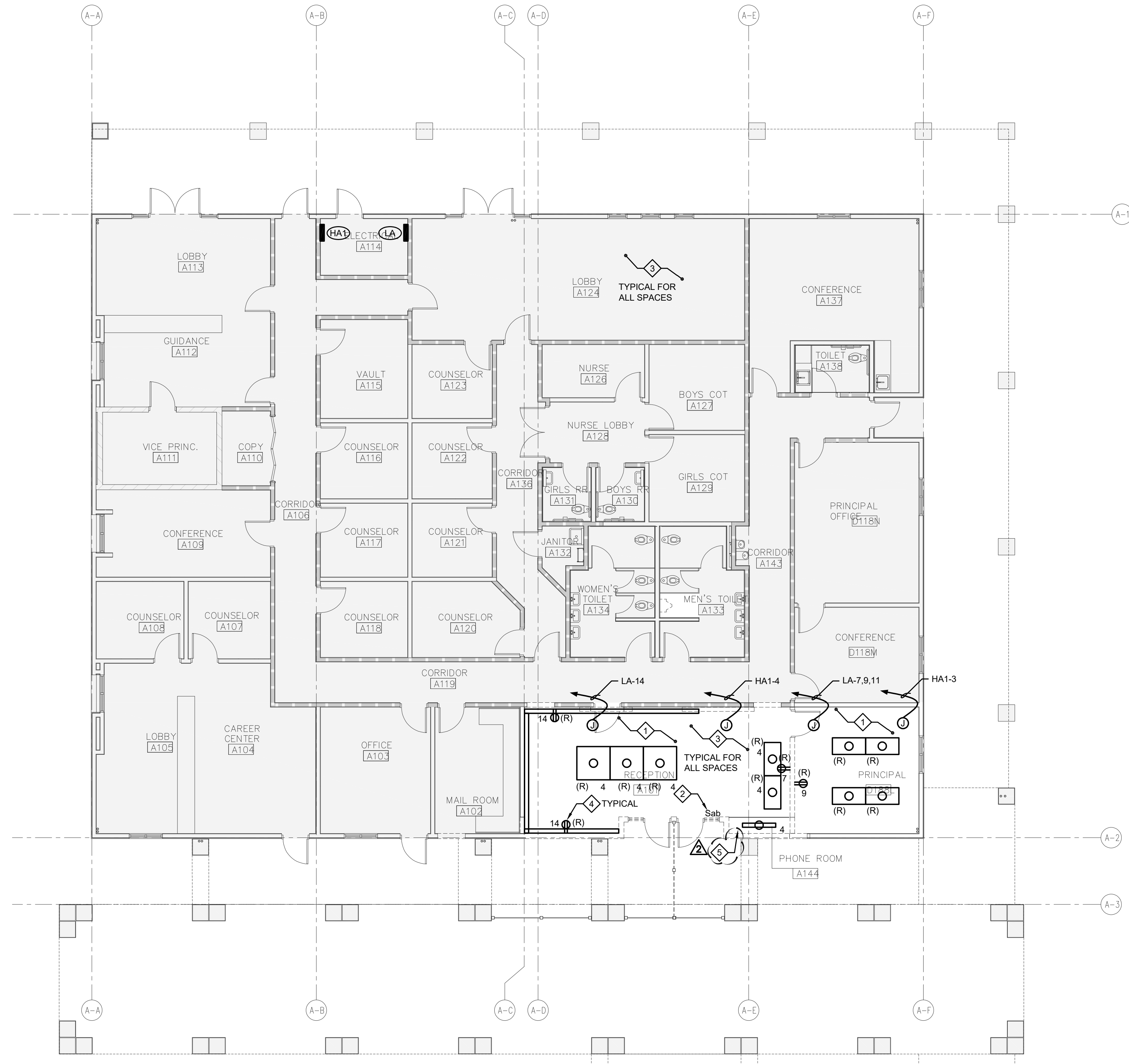
ELECTRICAL DEMOLITION FLOOR PLAN - BLDG A SCALE: 1/8" = 1'-0"
